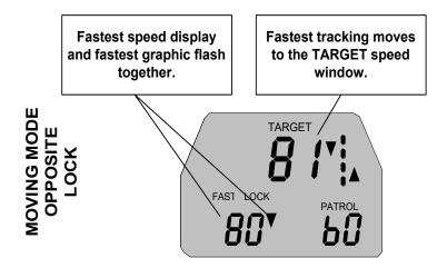
If the Lock button is pressed while tracking a fastest vehicle in any mode, the fastest speed will be locked in the LOCK window, and the fastest tracking will move to the TARGET window. After lock, both the LOCK window and the fastest indicator will flash together.
